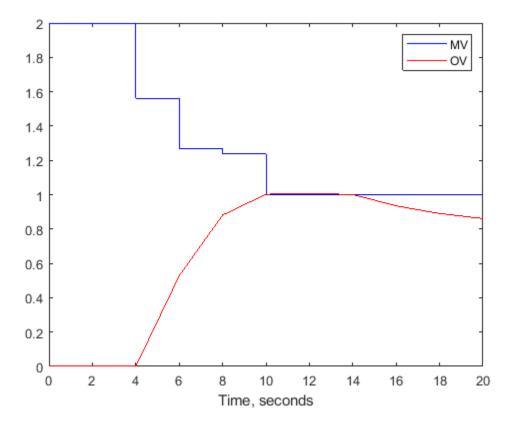
From the plot, you can observe that the original MV upper bound is active until t = 4. After the input delay of 4 seconds, the output variable (OV) moves smoothly to its new target of r = 1. reaching the target at t = 10. The new MV bound imposed at t = 10 becomes active immediately. This forces the OV below its target, after the input delay elapses.
